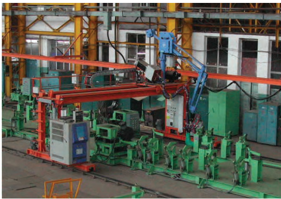
Side balaman welding line
