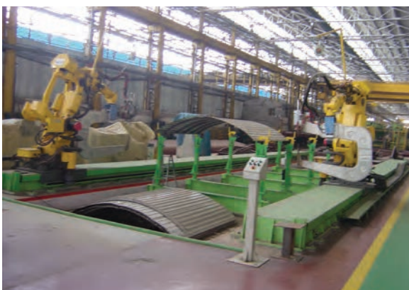
Roof robot welding line
