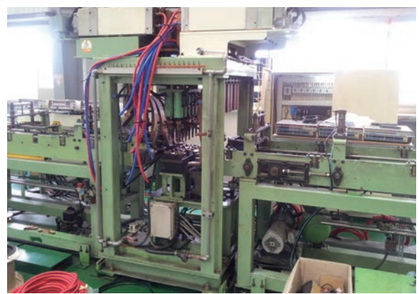
Radiator multi spot welding m/c
